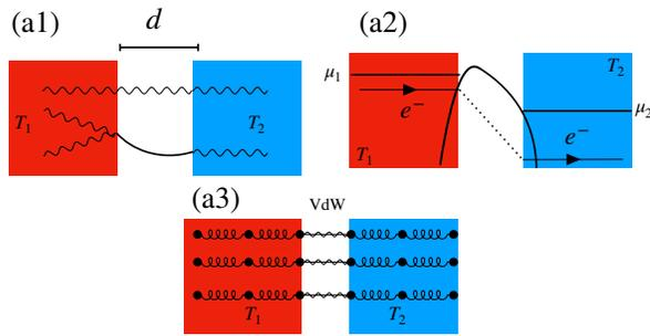
(a) Illustration of the different heat exchange mechanisms between two metals at temperatures  $T_1$  and  $T_2$  and chemical potentials  $\mu_1$  and  $\mu_2$ , respectively, for gap distances  $d \leq 1\text{nm}$ . (a1) Propagative and evanescent electromagnetic radiation (a2) Electron tunneling through electrostatic and image force potentials (a3) Acoustic phonon tunneling due to Van der Waals forces.
