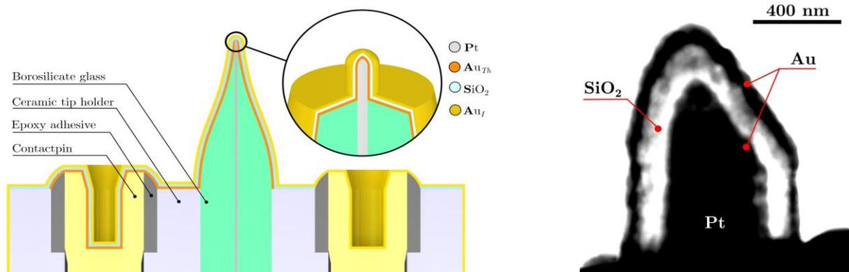
**Figure 1:** Structure and TEM image of a PASA-tip
