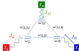
Fig. 2 : Quantum thermal transistor scheme made of three spin in interaction (spin ring model)
