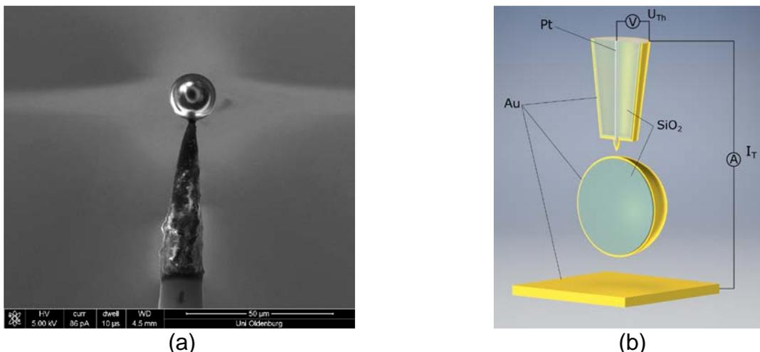
**Figure 1:** (a) Sphere probe during glue testing. (b) Schematic of a sphere probe without glue, not to scale.
