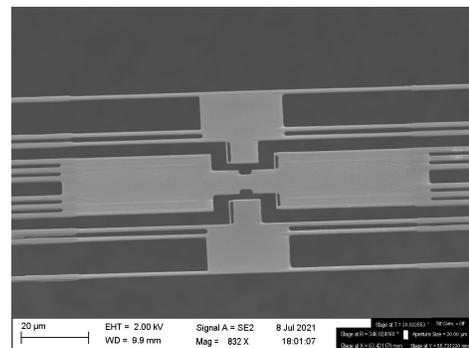
**Suspended thermometer, four terminal device.** On the left, there is a wide view of the device, the bridged membranes with beams are visible. On the right, there are four suspended membranes of SiN<sub>x</sub> with the platinum meanders on top, the two central membranes are connected to each other, while the other two side membranes are suspended individually by the beams. This is a scanning electron micrograph acquisition made in the laboratories of University of Basel.
