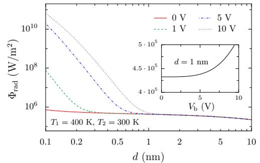
(b) Radiative heat flux between two semi-infinite gold slabs with respect to the gap thickness  $d$  for different bias voltages. Inset: Radiative heat flux as a function of bias voltage.
