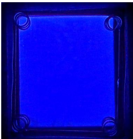
Fig. 1: Image of the plasma generated using the novel electrodes in presence of a catalyst.
