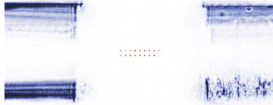
FIG. 1: Superimposed image of the scattering fiber cavity [left and right] illuminated by fluorescence beams, and a mean background-free image of the atom array [center].
