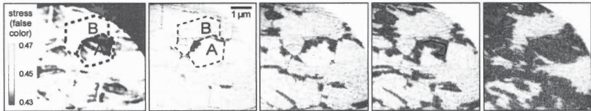
Fig.1: Growth sequence of CuPc/gr/Ir(111): The first image shows the clean gr/Ir(111) surface in false colors, dark areas corresponding to less, bright to more strongly stressed regions. In the following images CuPc crystallization is first observed on relaxed regions "A", and only subsequently on stressed regions "B".
