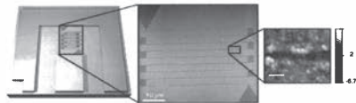
FIGURE 2 : AFM image of HTSc meanders made by ion irradiation embedded in a CPW line
